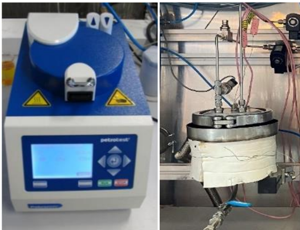
Figure 6: Standard test method "PetroOxy" and reactor in "BigOxy" test rig
