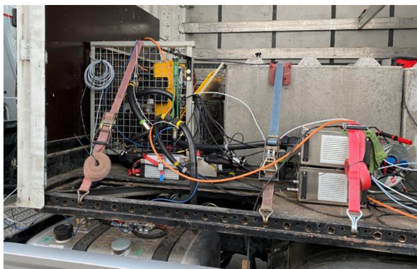
Figure 3 PEMS installation in the vehicle trailer bed
